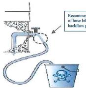
Recommended installation of hose bib vacuum breaker backflow preventer
