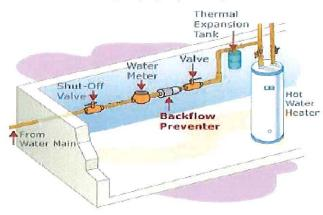
Many industrial and commercial customers on use water in manufacturing, in their heating or cooling system, or for other non-drinking uses. These customers are required to install a "backflow prevention device" where the water enters their building to prevent any possible contamination of the water mains. These devices are tested annually to make sure that they are working properly.
